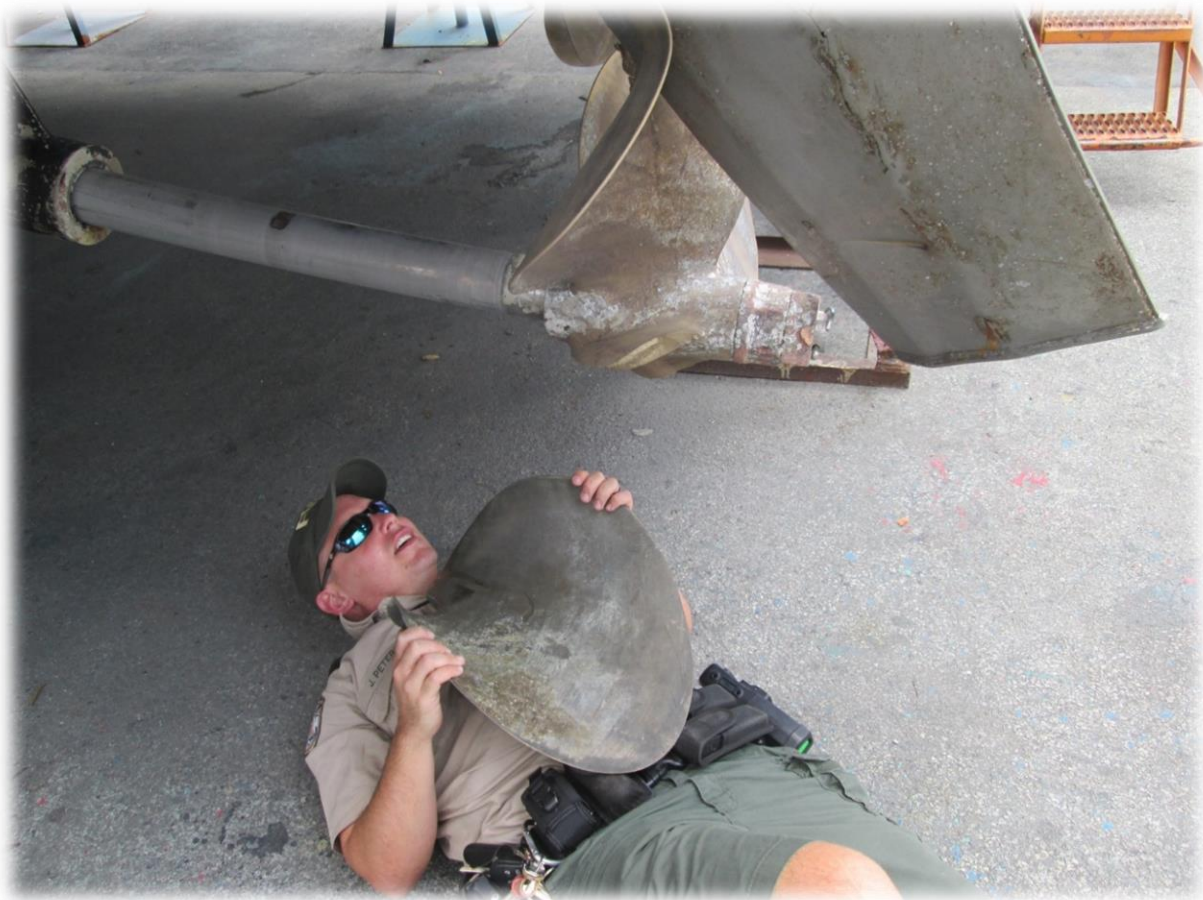
Photo detail: Matching a broken propeller blade to a vessel that had struck a coral reef and had not reported the accident. The blade was recovered from the coral reef and brought to the marina where the vessel was being repaired to confirm the vessel was the one involved in the boating accident and coral damage.
